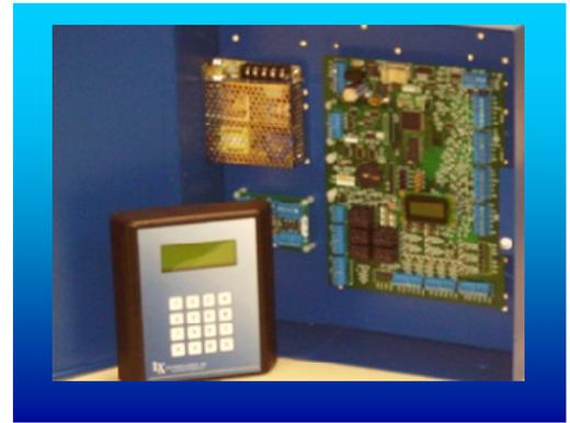
The IAD-4514 provides real time control and processing for access control, alarm reporting and remote control operation in the security environment. The IAD-4514 has four high-speed communication ports and comes standard with 4 MB Ram (Expandable to 16MB). The IAD-4514 supports interfacing with four card readers, 14 supervised inputs, and 5 outputs to provide access control at two doors with two readers or at four doors with an individual reader at each door.
